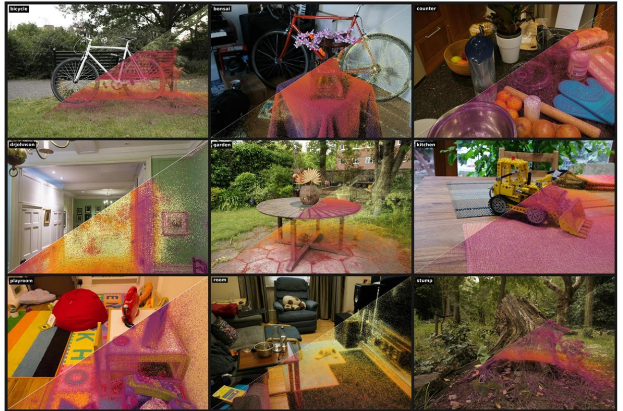
Fig. 7. Images from the real-world test cases (described in Sec. 5.1), with point sets projected to illustrate the density and spatial spread of the data. The scenes span a range of indoor and outdoor environments with complex spatial distributions and point counts ranging from 2M to 4.2M.
